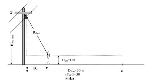
Figure 1 – Illustration of Slant-Range Distance
